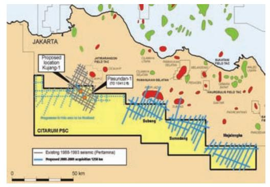
Figure 2: Proposed 1250 km 2D seismic survey on Citarum PSC
